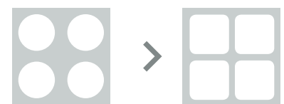
isotropic/anisotropic pore shaping
